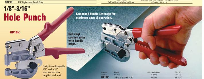
Does the work of more expensive bulkier punches faster and easier. Use in any edge application for making holes in window extrusions, metal ductwork or sheet stock. Compound leverage increases one hand mechanical advantage 8 to 1. Spring return handles allow quick set-up for repetitive applications. Stop gauge permits adjustments from 1/4" to 1-1/8"
