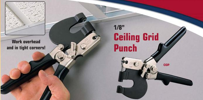
Malco's unique, Ceiling Grid Punch makes a clean 1/8" (3.2 mm) hole in up to three layers of 25 gauge (0.53 mm) ceiling grid. The tool's slim but strong steel "C" frame allows easy access in tight corners and is ideal for punching through main tees and perimeter wall angle that is to be secured with rivets. A generous throat opening allows full operation from the edge of both standard 1" and 1/2" (25.4 & 12.7 mm) grid
